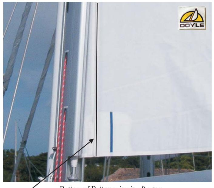
Bottom of Batten going in after top (vertical black line to illustrate batten location only, it is not on sail)
